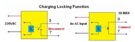
Charger provides a set of relay normally closed contact as charging locking signal output. When the charger has no electricity, the contact connects, while the charger connects to the AC power supply, the contact disconnects immediately. The rated current of contact is 1A, withstand voltage 30VDC / 250VAC.
