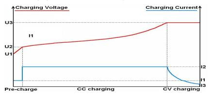
U1= $\frac{U3}{2}$ , U2= $n_{\rm fl}$  ×2.5V, U3=Maximum voltage for the battery pack I1= $\frac{I2}{2}$ , I2=Maximum charging current for the battery pack, I3= $\frac{I2}{6}$
