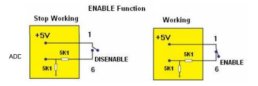
As for lithium battery charger, it's essential to use an enable signal to control the charger's work or close. Isolated circuit (such as Relay or Optocoupler) shall be adopted to control the charger's work or close. Note that if the control circuit is not independent, it lead to damage of the charger.
