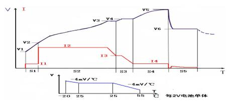
current charging I1, finally, the pre-charging process is completed when voltage rises to U2.
